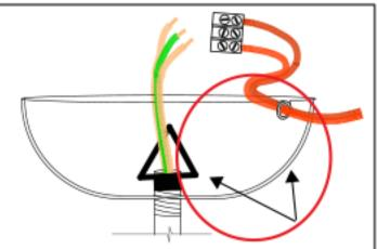
Place the plug-in kit ceiling cap with cord inlcuded over the central threaded pipe of the chandelier. Secure the cap to chandelier by screwing on the triangle bolt.
