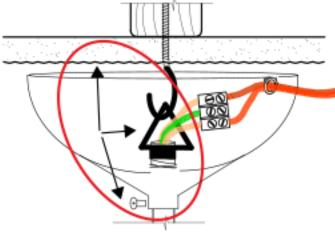
Hang chandlier on hook with triangle bolt. Push celing cap flush to the ceiling then tighten the small side screw to keep cap in place.
