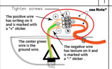
\*Note: The plug-in cord connector may be marked with "L" for Positive and "N" for Negative. If there are no markings on the connector or cord, then it doesn't matter which cord goes to positive and negative wires on the chandelier. There is no ground wire on the cord. 3
